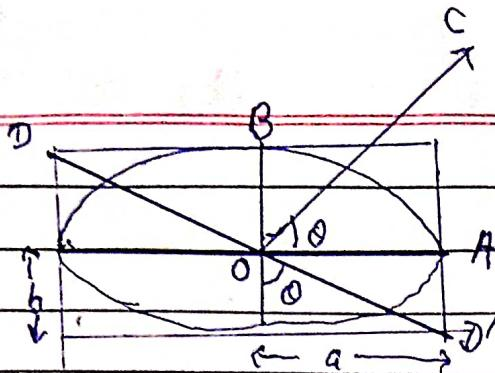
discussed above. The reading of analyser  $N_2$  is noted. Let OA and OB represents optic axes of prism of compensator. OC represents the direction of main cross-section of  $N_2$  while DD' represents plane of vibration of light at the cross-wire.
