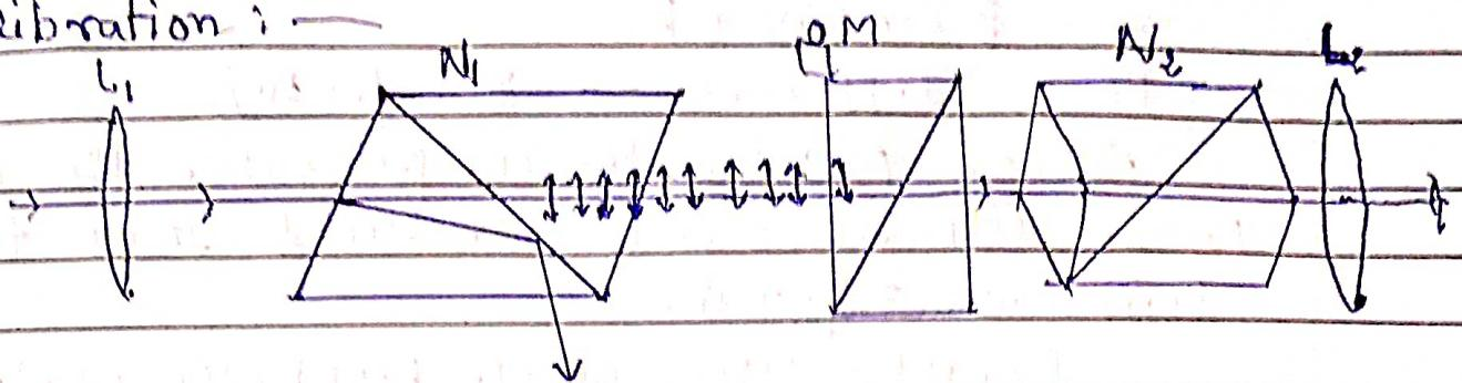
To calibrate micrometer screw M, the compensator C is kept between two crossed nicols N<sub>1</sub> (Polariser) and N<sub>2</sub> (analyser).
